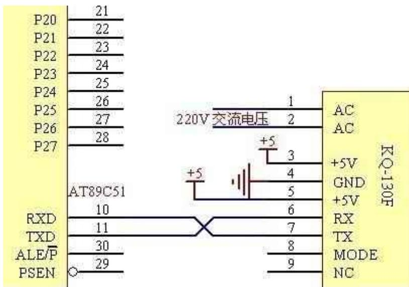
KQ-130F power line carrier data transceiver module and the microcomputer 9 pin RS232 port connection FIG:
