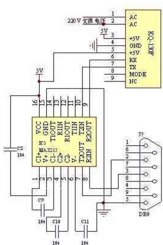
KQ-130F power line carrier data transceiver module after the microcomputer of FIG. 9 pin RS232C serial debugging assistant connection test pattern:
