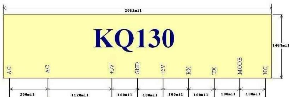
1P-AC: Firewire (or neutral) AC voltage 220V
