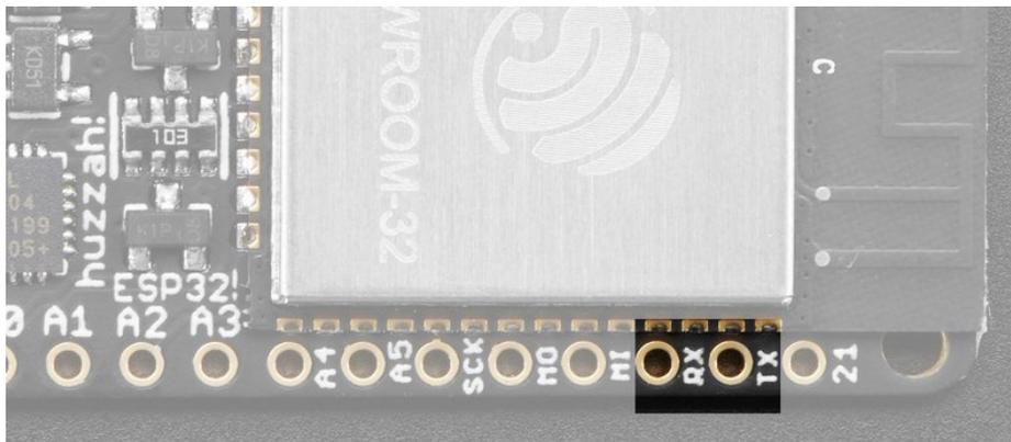
The TX pin is the output *from* the module. The RX pin is the input *into* the module. Both are 3.3V logic
