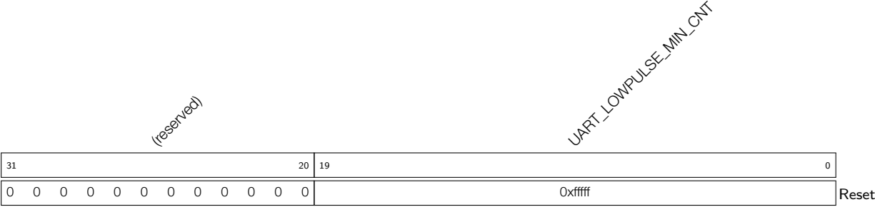
Register 12.17: UART_LOWPULSE_REG (0x0028)
