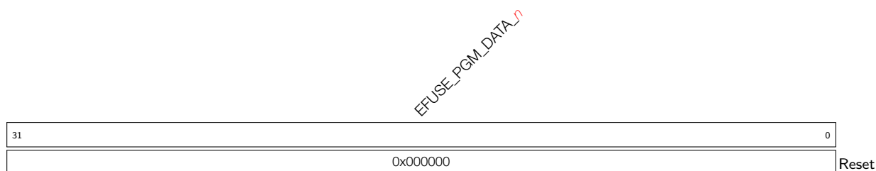
Register 16.1: EFUSE_PGM_DATA n _REG ( n : 0-7) (0x0000+4* n )
