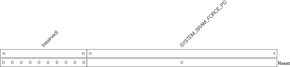
Register 5.4: SYSTEM_SRAM_CTRL_1_REG (0x000C)
