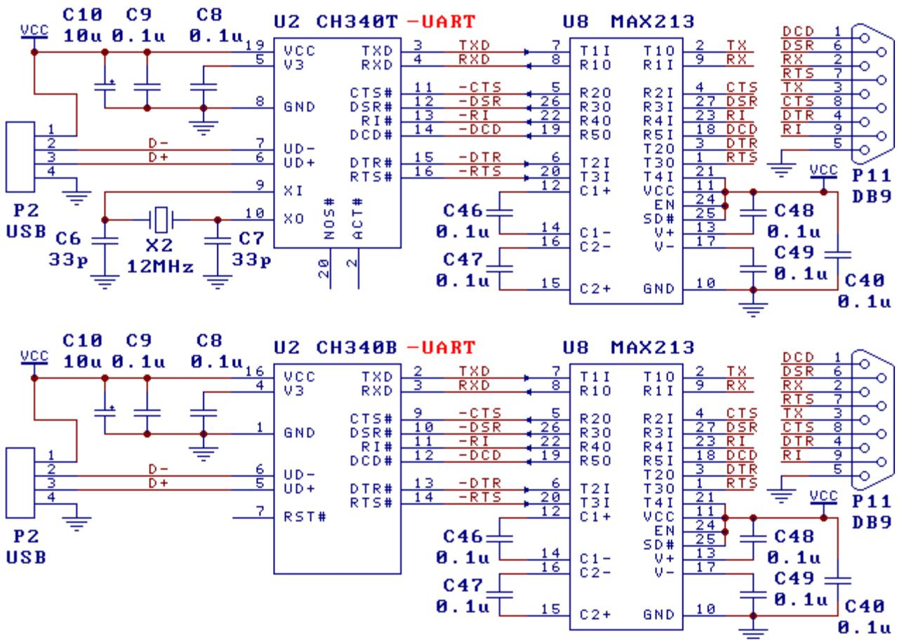
The figure is achieved by CH340T or CH340B (or CH340C) USB to RS232 serial port. CH340 provides a common serial signal and MODEM signals, by the level conversion circuit U8 is converted to TTL serial RS232 serial port DB9 pin P11 is the same as the ordinary and the pin 9-pin serial port of the computer functions, a similar type of U8 there MAX213 / ADM213 / SP213 / MAX211 and so on.
